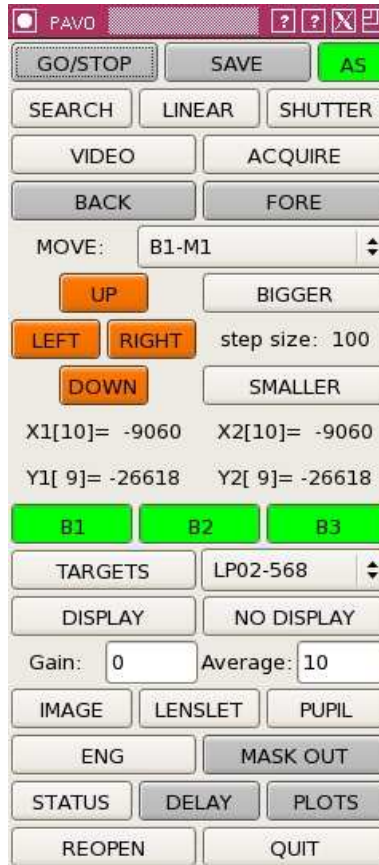
Figure 5.2: The PAVO GUI used to control the instrument. Green indicates that a button is active. In this screenshot, autosave is turned on and the B1, B2, B3 shutters are open. The camera is off; the [GO/STOP] button will turn green when the camera is on. The mask is in (the [MASK OUT] button will turn green when the mask is out).
